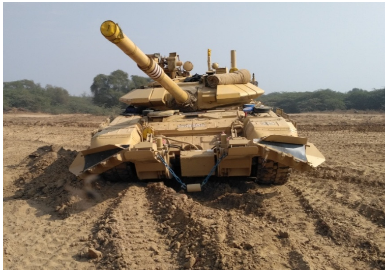
T-90 Tank fitted with Mine Plough
